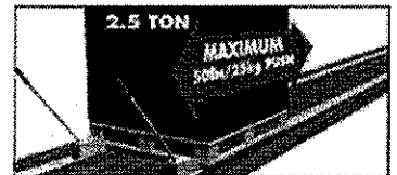
The load is now 'live' and free to be pushed the length of the truck
